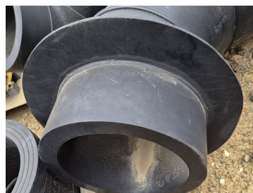
500 mm ID HDPE suction elbow with its sharp entry edge.
